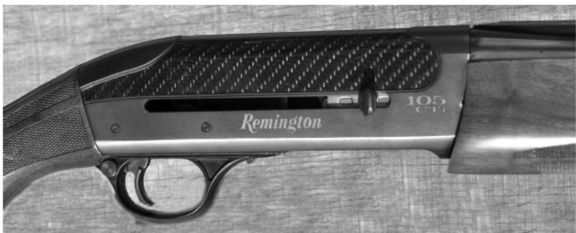
Above: The bolt handle on the Remington 105Cti is alone on the right sidewall of the receiver; there is no ejection port since the gun is a bottom-ejection model.
