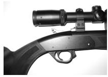
Despite the use of high rings, the Knight Shadow had inadequate hammer to scope clearance to easily cock the gun, particularly with gloved hands.
