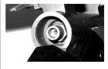
The Knight breech plug was comparatively filthy, allowing 209 primers to spit their material all over the inside of the breechplug area and action. The breechplug was positioned way too far inside the barrel.
