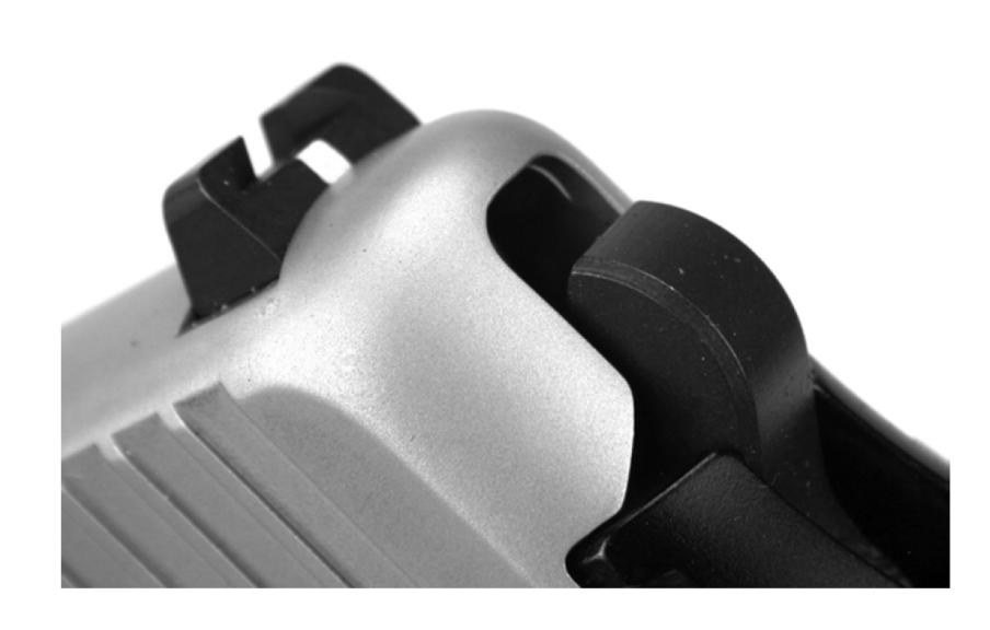
With the action cocked, the hammer stood back from the firing pin. The rear of the slide was beveled. The front sight had a tritium dot, but the rear sight featured a single-line notch. This amounts to one-half of the Siglite night sight package.
