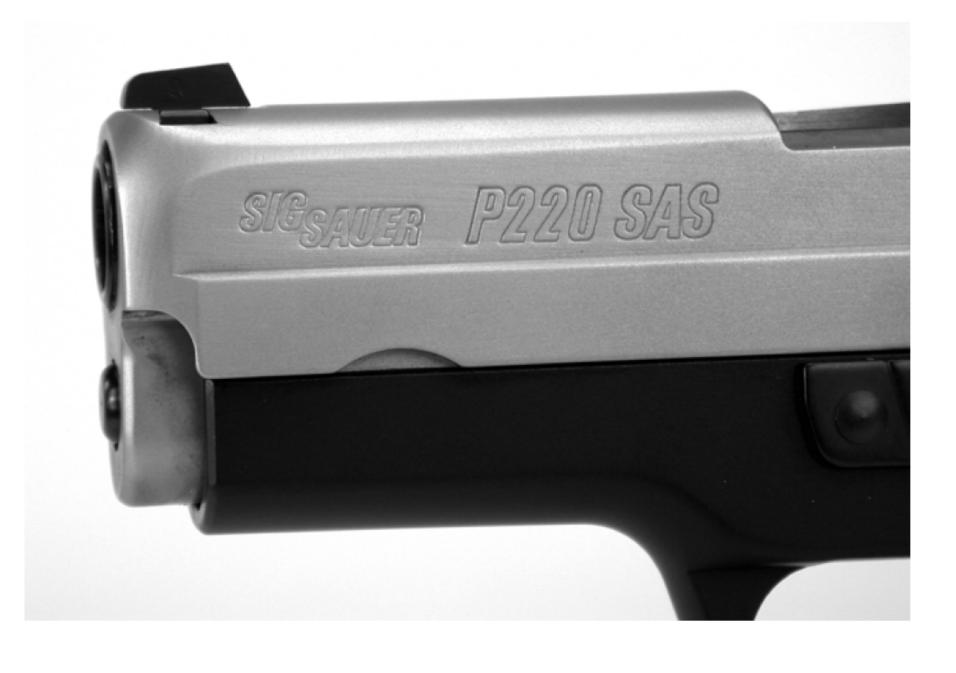
Beveling, or dehorning, the front of the slide is part of the SAS package. Note the absence of an accessory rail on the frame underlug. We think this model favors concealed carry.
