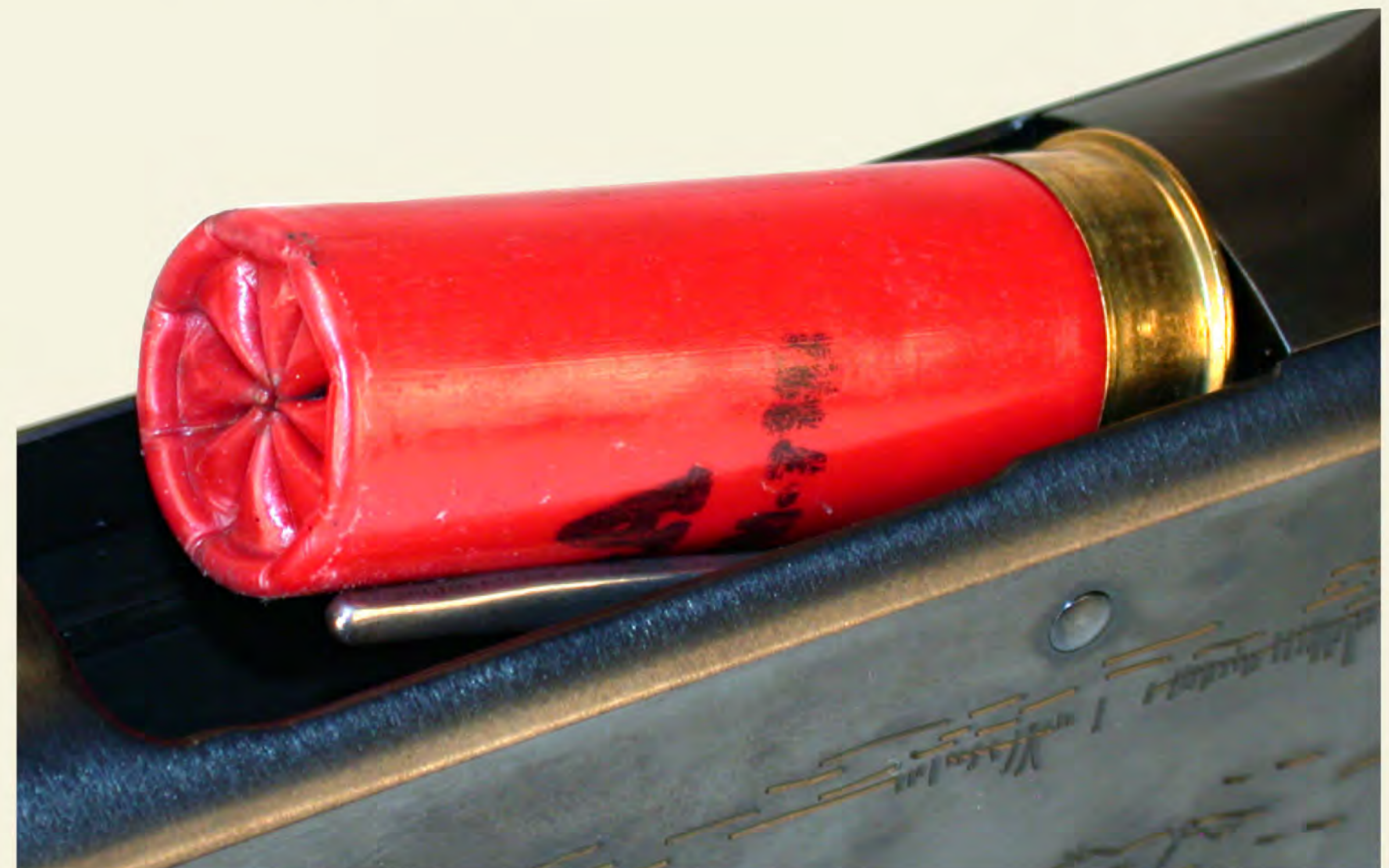
Above: Single loading began with placing the round atop the elevator. Working the slide to drop it down and send it forward into the chamber was more reliable when performed in two distinct movements. But single loading was easier still when fed from the magazine.
