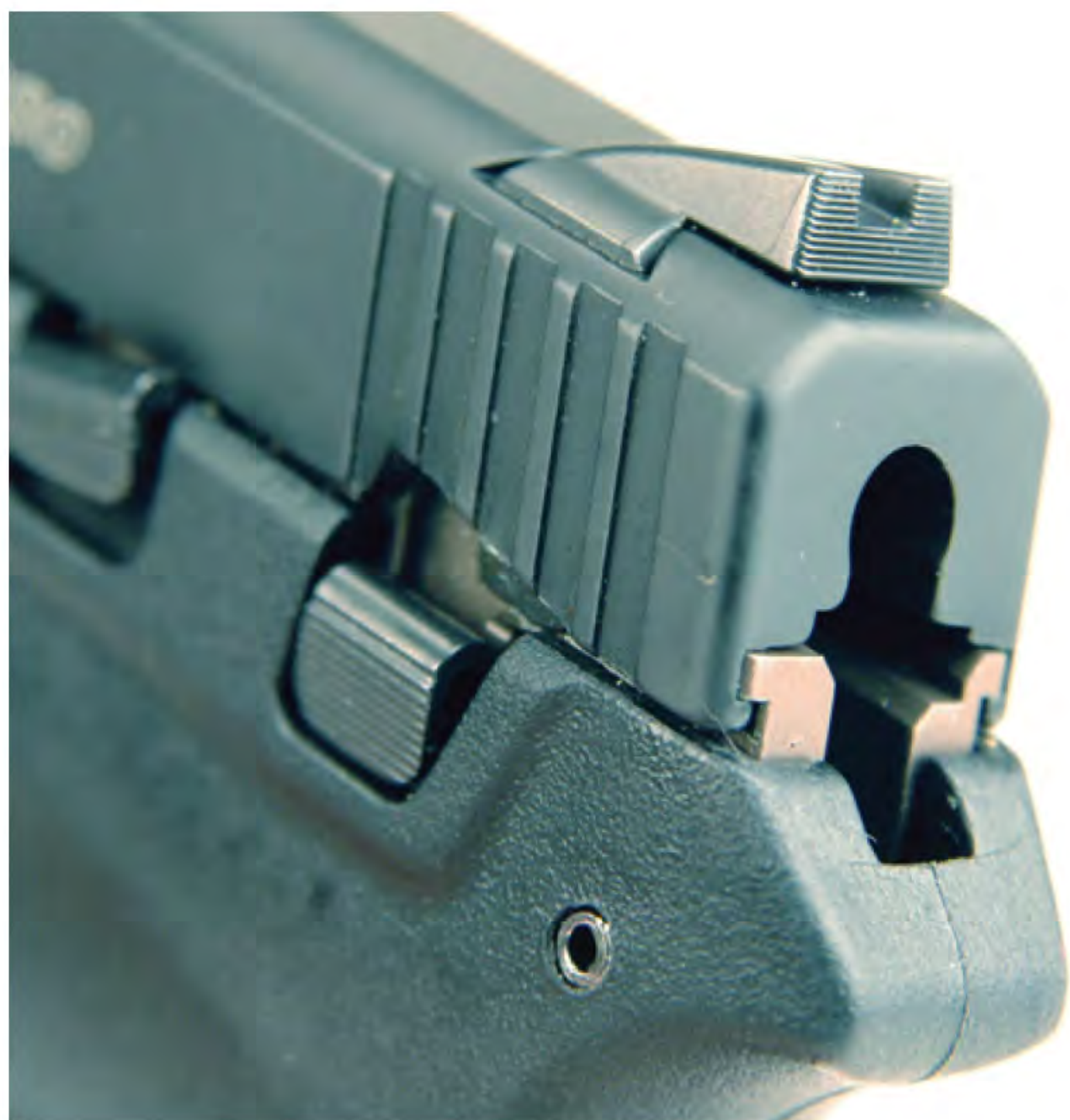
Above: The rear sight was a miniature reproduction of a popular target sight. The sight picture was vivid beyond its scale, in our view. Note the heavy molded look to the frame.
