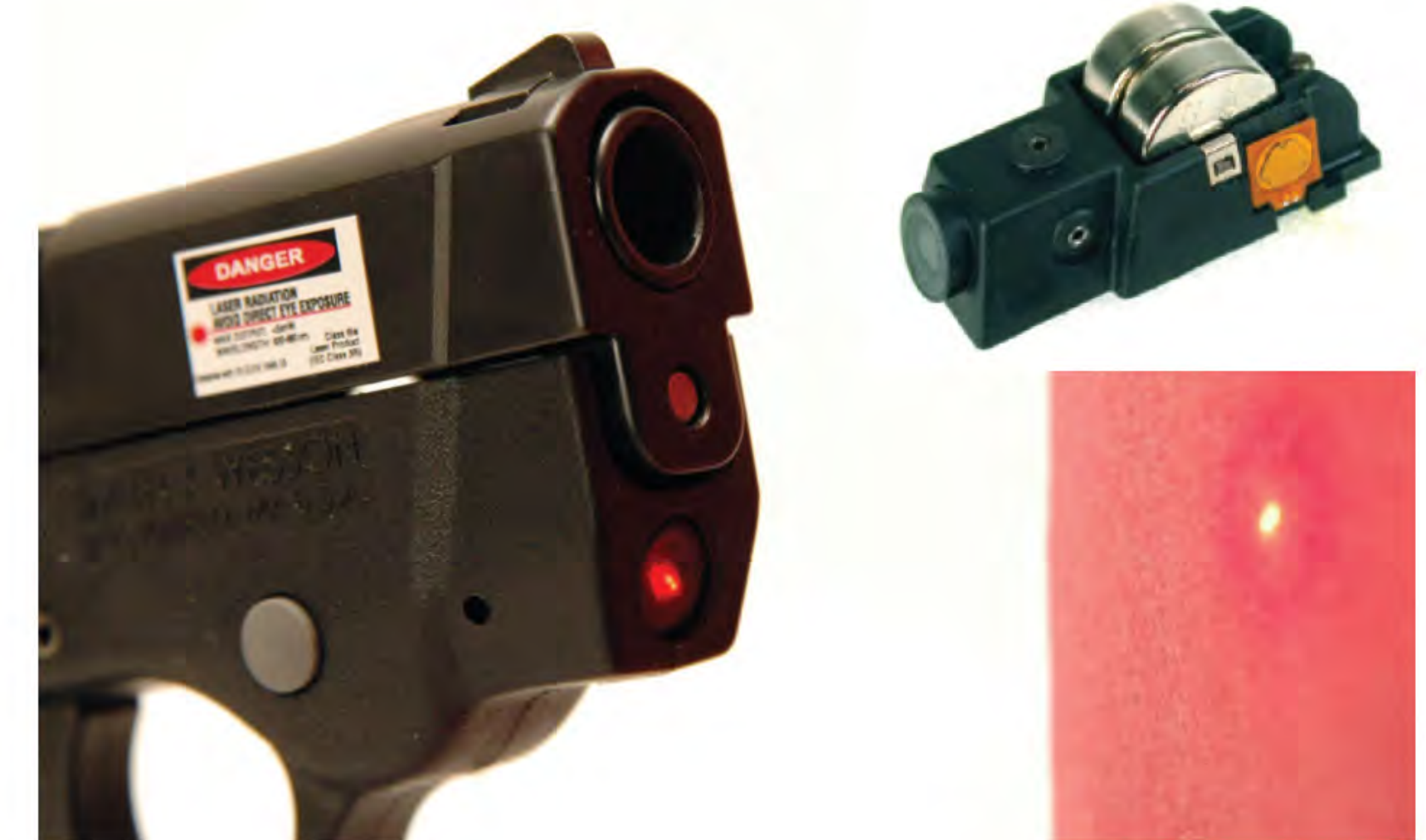
Above: The laser was controlled by membrane-style buttons found on either side of the frame. Press once for a solid beam and twice for a pulsing, strobe effect. Pressing a third time turned the unit off. Top right: The integrated laser (by Insight Technologies) was powered by two No. 357 batteries.
