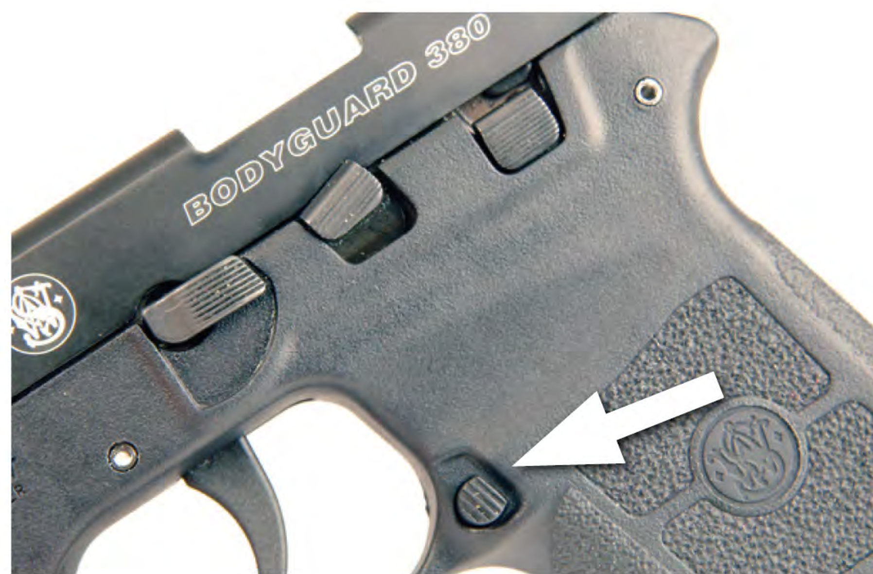
Above: Right to left, the thumb safety, slide stop, and takedown latch were positioned along the left side of the frame. The magazine release, arrow, was shielded from unwarranted contact by a ridge and a heavy detent spring. Somewhat heavier than its competitors, the Bodyguard felt rigid in the hand.
