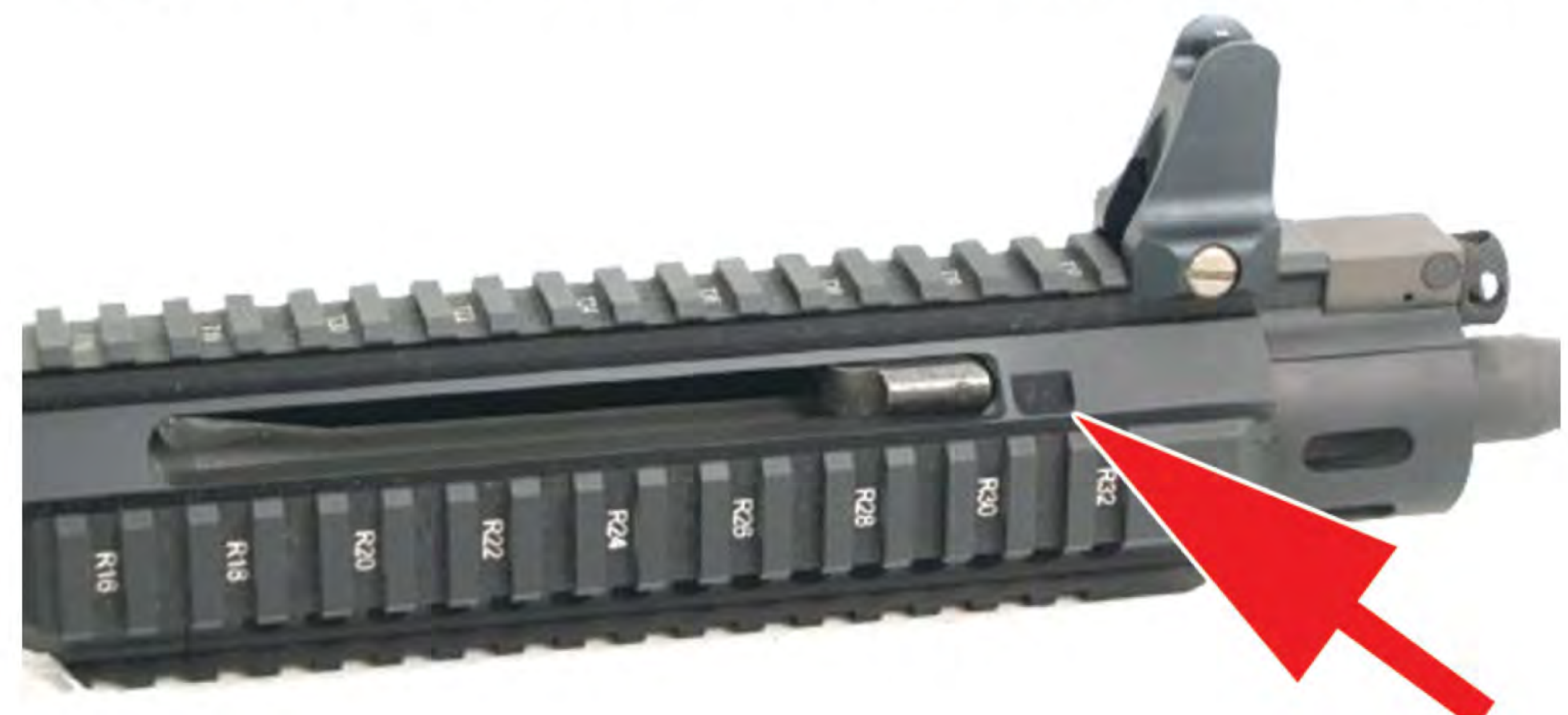
Above left: The ambidextrous forward-placed charging handle/forward placed assist (arrow) permits the operator to charge, clear, or forward assist the weapon with the front hand. The operator pulls the handle to open the action. Right is the opposite side of the handguard and the forward charging handle. The arrow points to the retention notch, which accepts the folded-in handle when it's reversed.
