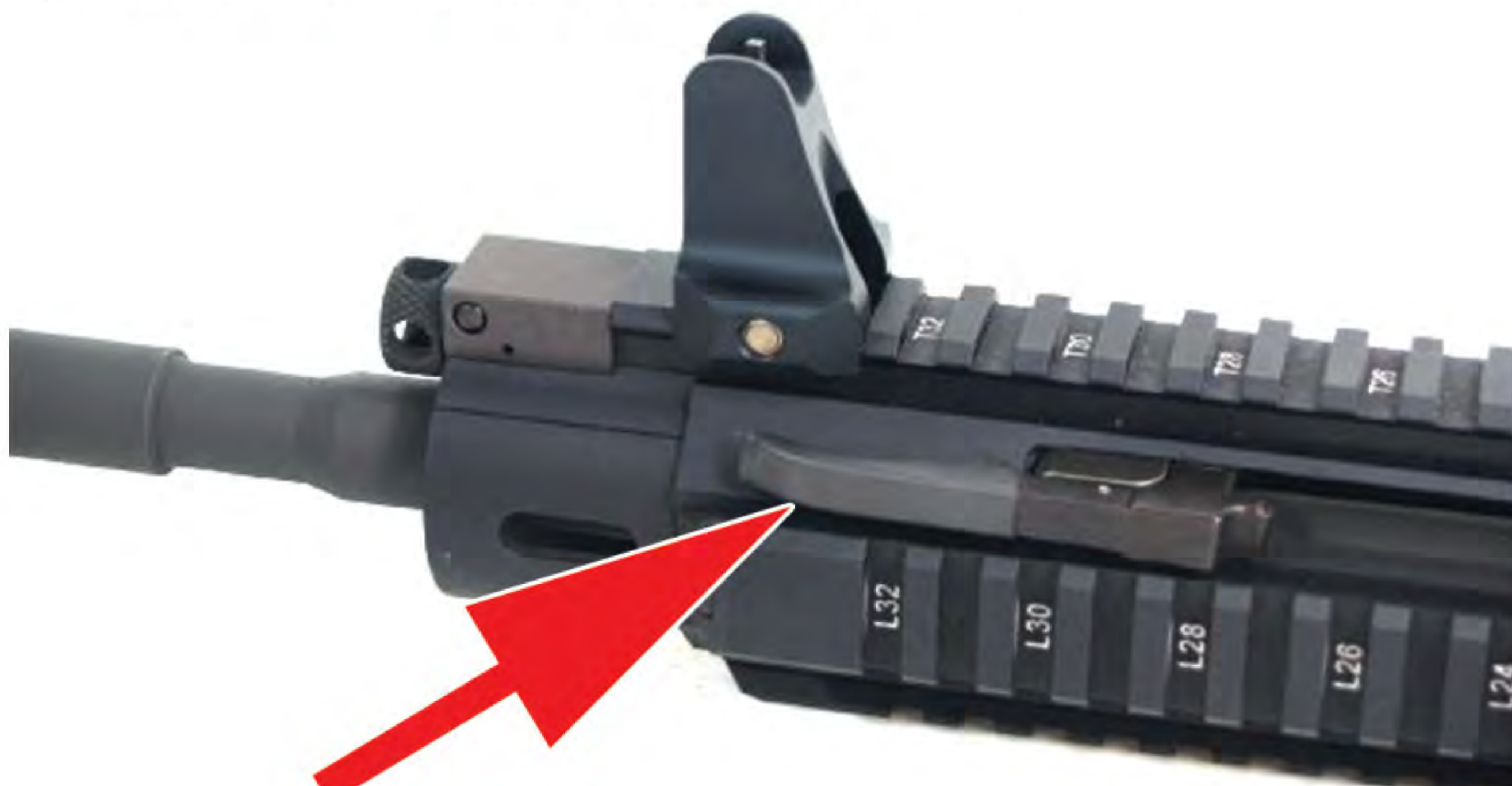
Above left: The ambidextrous forward-placed charging handle/forward placed assist (arrow) permits the operator to charge, clear, or forward assist the weapon with the front hand. The operator pulls the handle to open the action. Right is the opposite side of the handguard and the forward charging handle. The arrow points to the retention notch, which accepts the folded-in handle when it's reversed.
