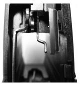
Here's a close-up view of the sear-release lever after it is lowered using the backstrap tool.
