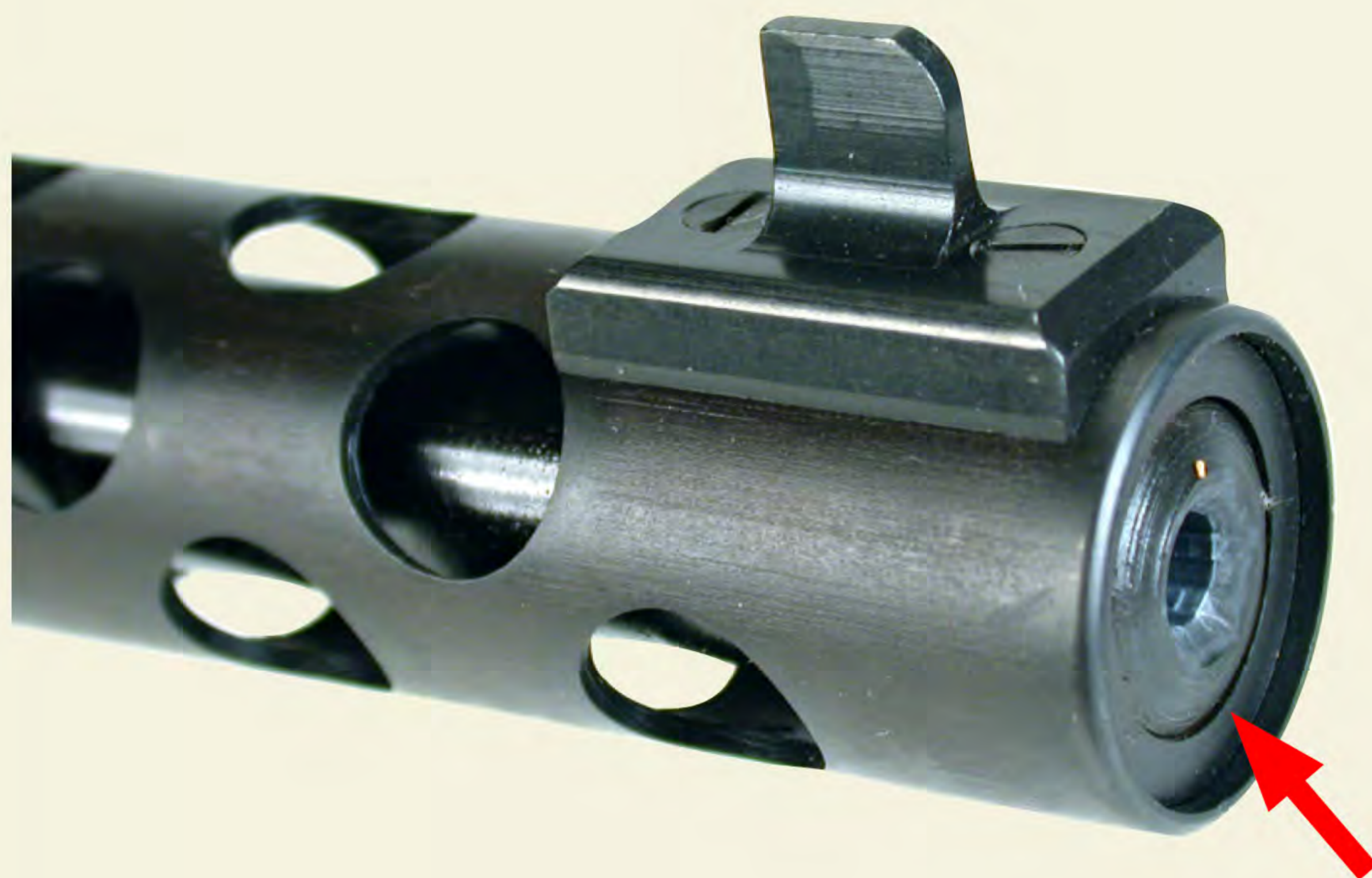
Above: The front sight was nothing fancy—just a tall post machined from polymer and screwed into the barrel cover. But it was precise and clear. Note the barrel support at the muzzle.
