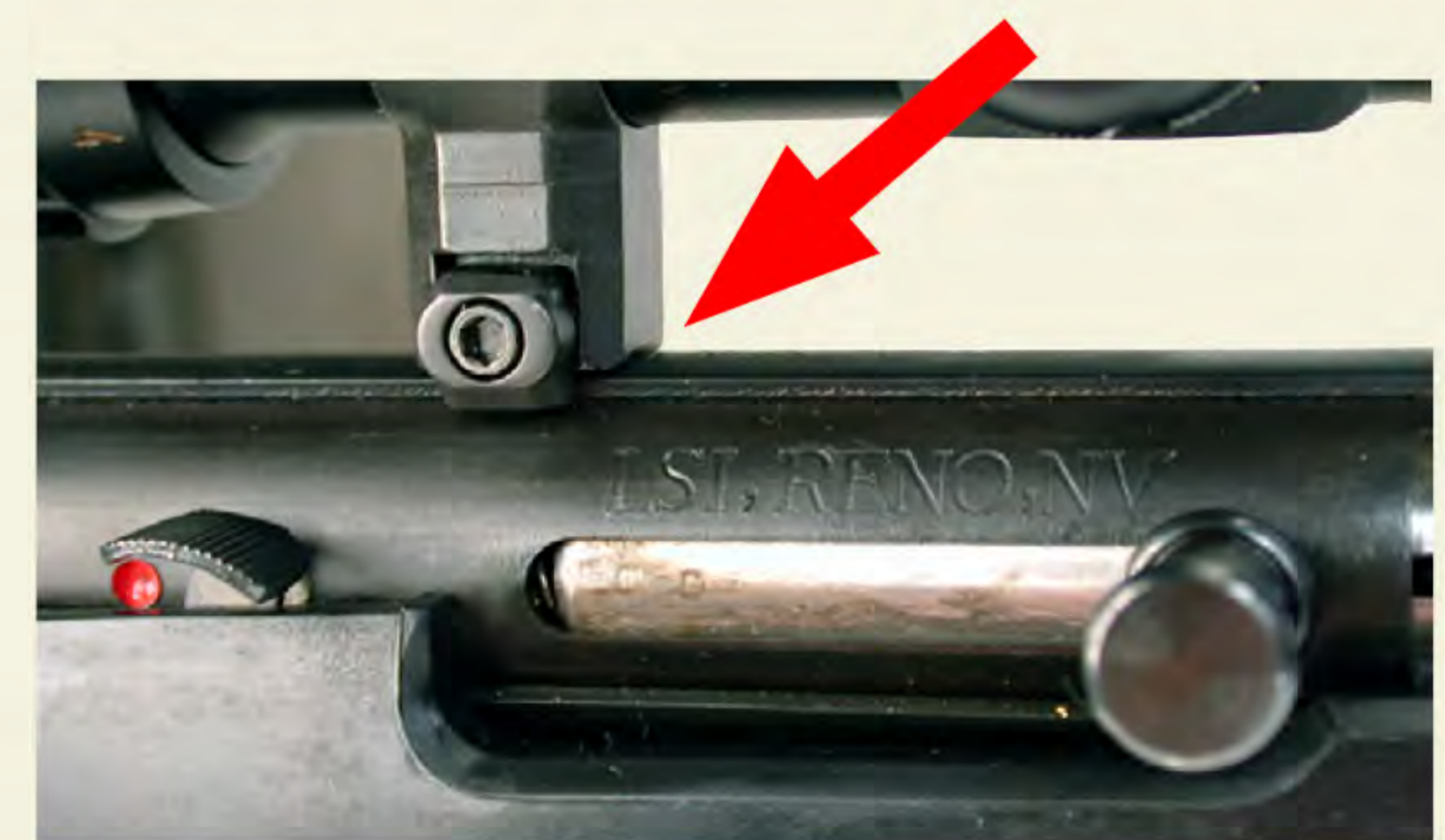
Right: Legacy Sports of Reno imports the Puma rifles from Italy. The receiver carried a 3/8-inch rimfire mount groove (arrow). To the left of the ejection port was the modest safety lever. The bolt handle was enhanced with roller action.
