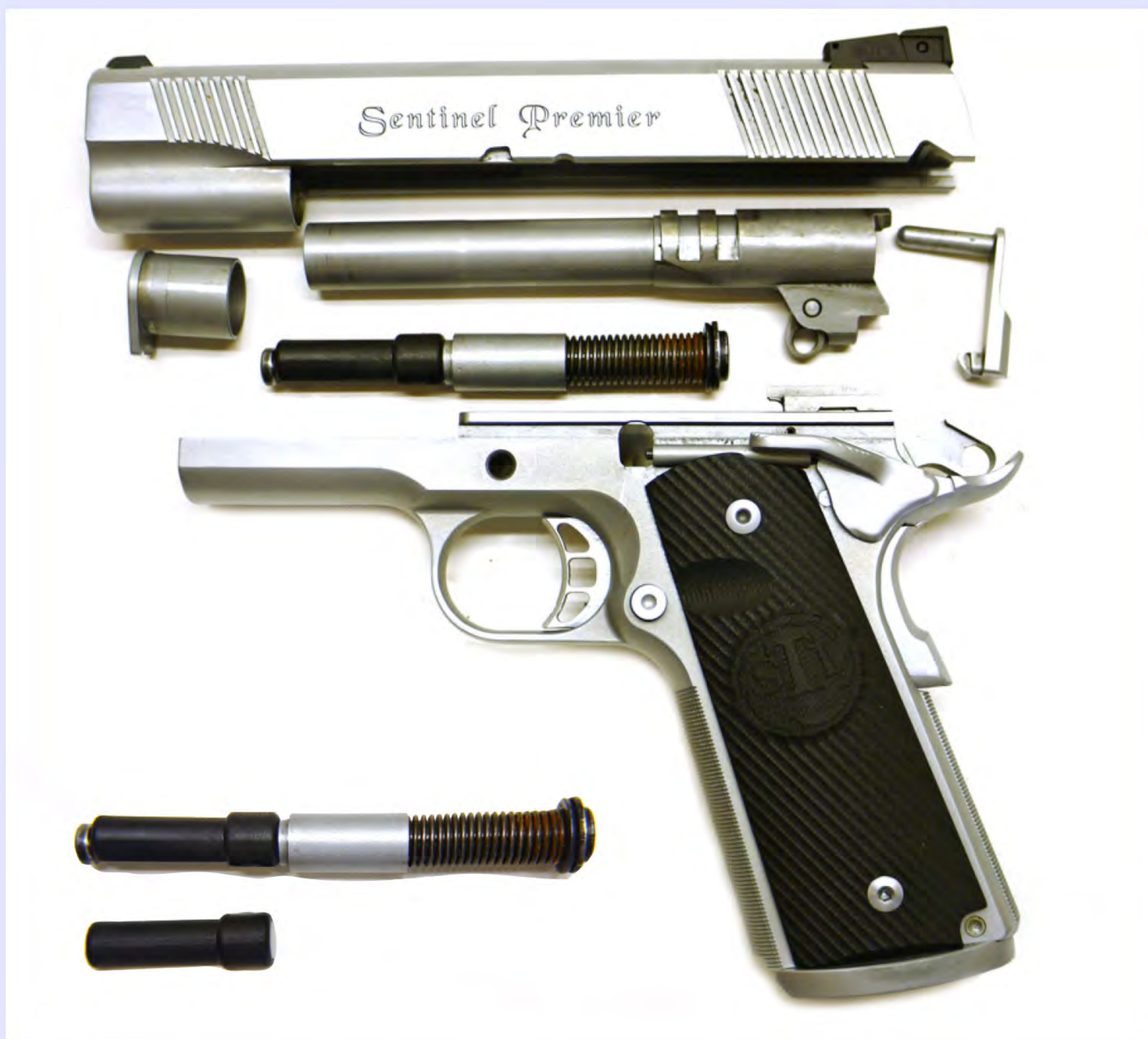
Above: The STI has a ramped, fully supported barrel held in a place by a match-grade bushing (inset, arrow). The muzzle was crowned to fit flush.
