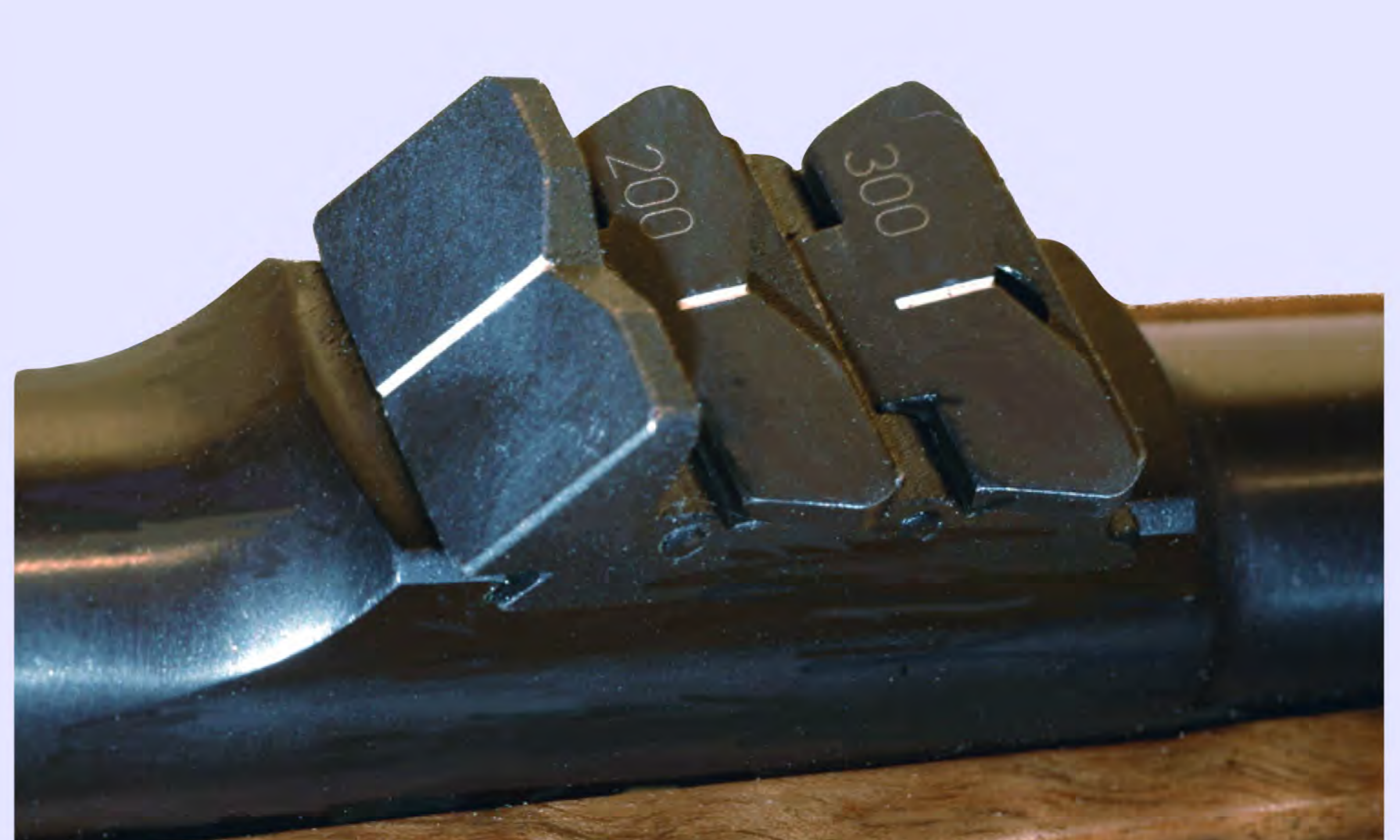
Above: Prominent center lines on the standard and the folding leaves let the shooter's eye line up the front bead faster and easier. The front sight was mounted in a ring that wrapped the barrel, and the rear was dovetailed into an integral base on the barrel. We liked this setup.
