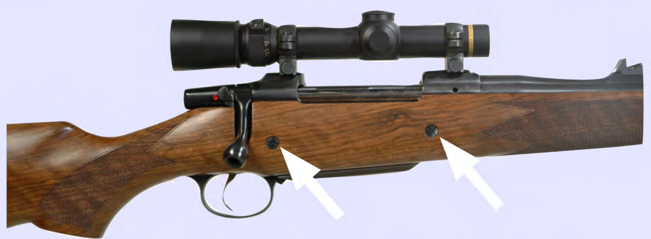
Above: Two crossbolts (arrows) helped keep that nice wood from splitting. The checkering was at least as good as that on the Kimber. The bolt would benefit from lapping, or use, to make it slicker. The 1.5-5X Leupold was about right for this rifle.
