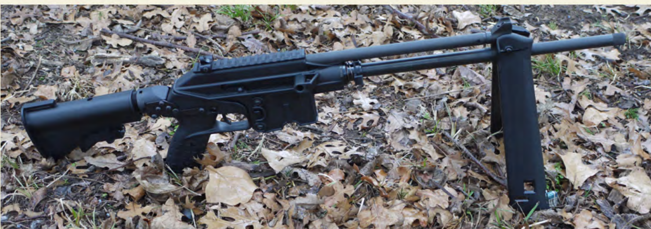
Left: The forend of the SU-16A opens up to become a bipod.
