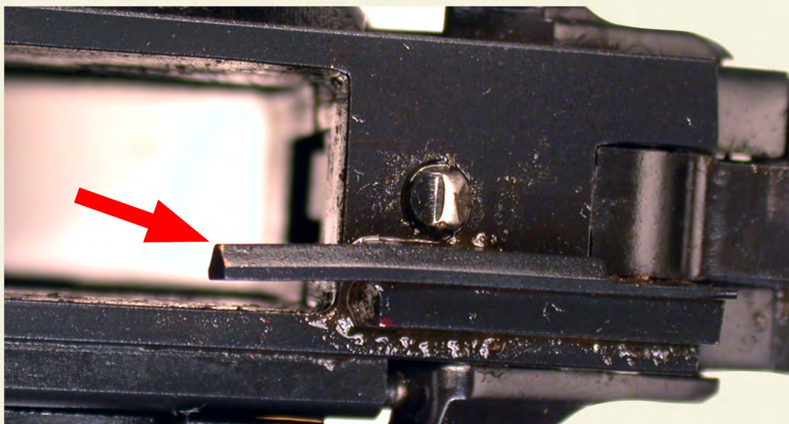
Above: The ejector on our STI Duty One, left and detail, below , was much longer than those found on either the Kimber, right, or Springfield Armory pistol, center. After suffering malfunctions, we returned our Duty One to STI for warranty service.
