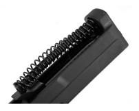
The polymer guide rod looked flimsy, bowing under the push of the recoil spring. But the P32PK was the only pistol in the test to run without a single malfunction.
