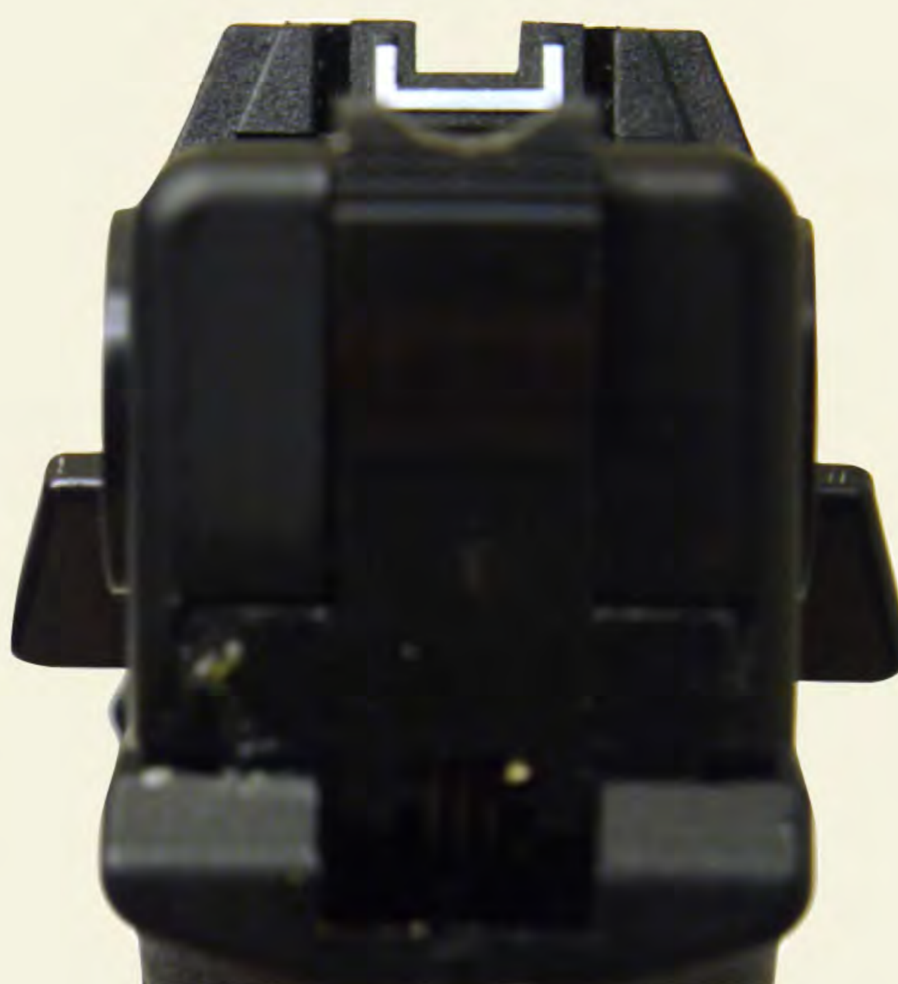
Right: Sights consisted of a white rectangle on the front, with an adjustable rear sight that was framed with a squared-off white line (shown). The sight picture was easy to access and was judged the best out of our trio of contestants.
