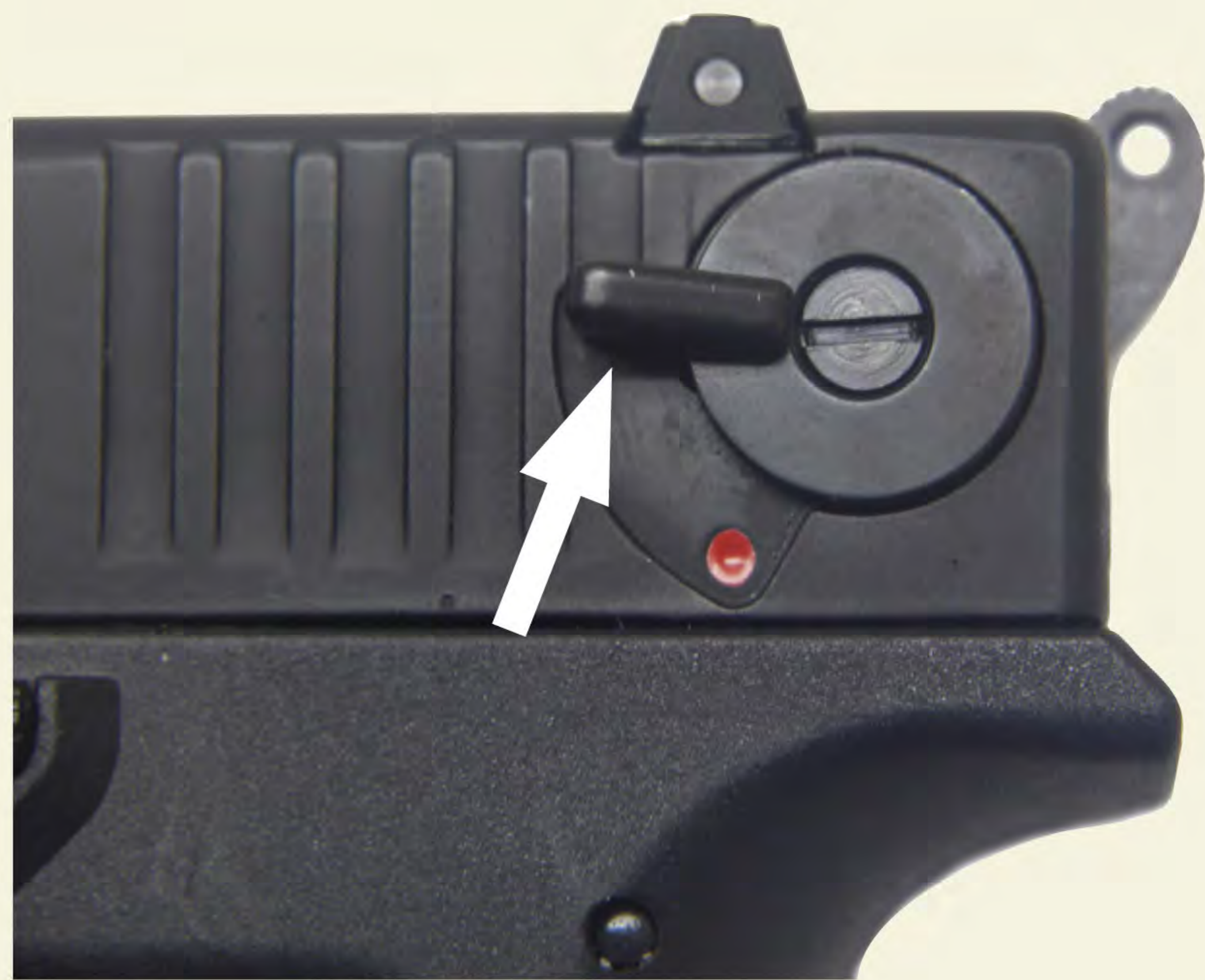
Right: The ISSC's ambidextrous decocking levers worked, but were a little awkward to operate.
