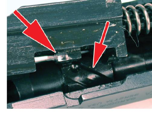
barrel. Driven by reciprocation of the slide they acted like a set of gears to turn the barrel.
