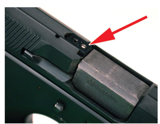
A pop-up chamber indicator was added to the slide. Shown here the chamber is empty.
