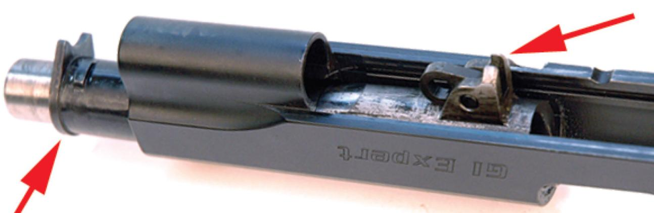
To dissassemble, after removing the spring and guide rod we rotated the Para's barrel bushing (left arrow) counterclockwise and pulled it from the slide. Then rotate the barrel link (right arrow) out of the way so the barrel can be slid through the front of the slide. No tools were required.
