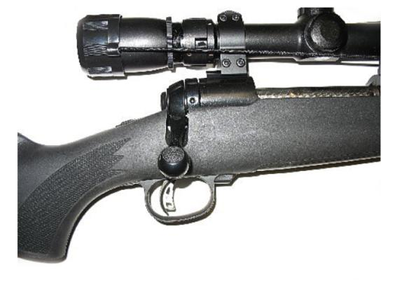
used in dense cover. The Marlin's bolt never did lock closed—it is easily snagged open in brush.
