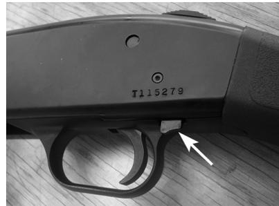
The receiver was aluminum, which helped keep weight down. We could work both the safety (arrow above) and the slide release (right, on the other side of the gun) without changing the shooting-hand grip and without having to dismount the
