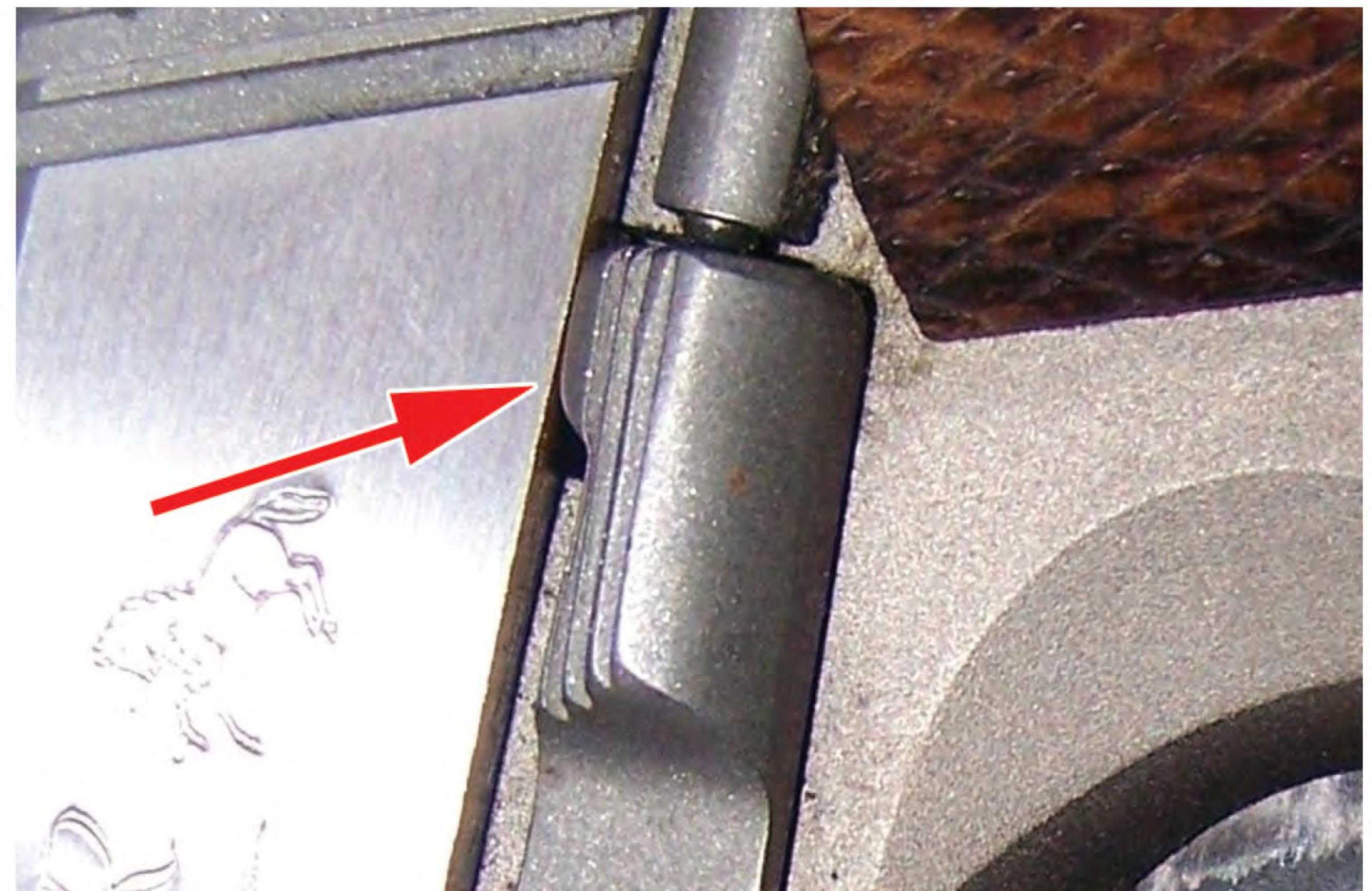
A slight disadvantage of an aluminum frame is that they are easier to damage than a steel frame. Do not allow the slide stop to snap into place after reassembly, but rather baby the frame when disassembling aluminum-frame 1911s.
