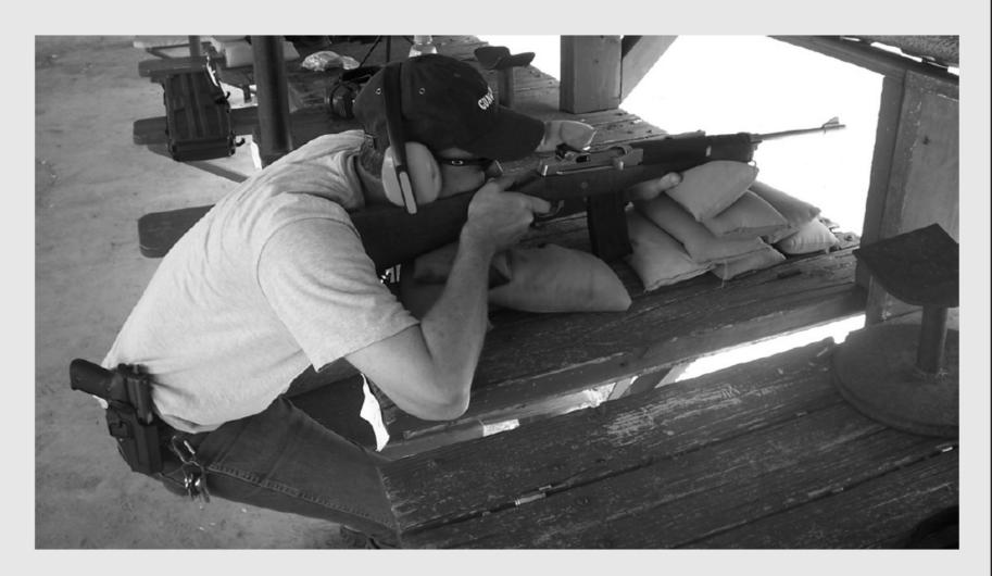
Shooting accuracy groups off the bench can be challenging when 30-round magazines are in play. Here, Test Coordinator K. R. Huey has constructed an elevated rest with sandbags under the forend and under the buttstock. That raises the boreline high enough to clear the high-capacity Ramline magazine.
