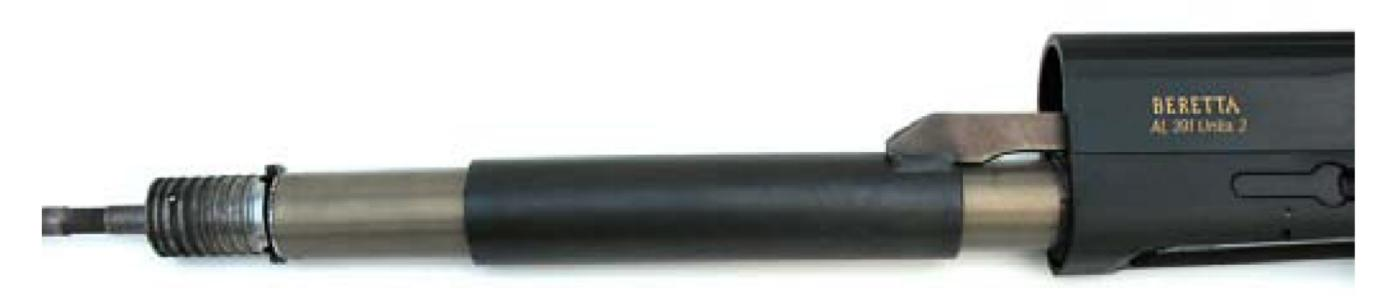
This latest version of the 391 action features Beretta's spinning, toothed gas piston. Beretta says that this allows the Urika 2 to go 50% longer between cleanings than ever before. We don't disagree; we've already put more than 1000 rounds through this Urika 2 without a thorough cleaning, and we have yet to have a single malfunction.
