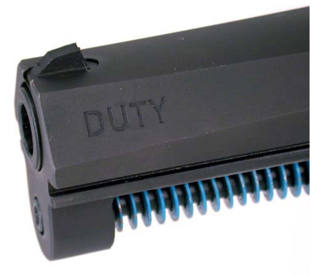
The top end of the P-07 was machined from barstock steel and featured unique sculpting to save weight. The flat wound recoil spring was long and powerful, demanding extra attention during assembly. The front sight was press-fit from the front of the slide.
