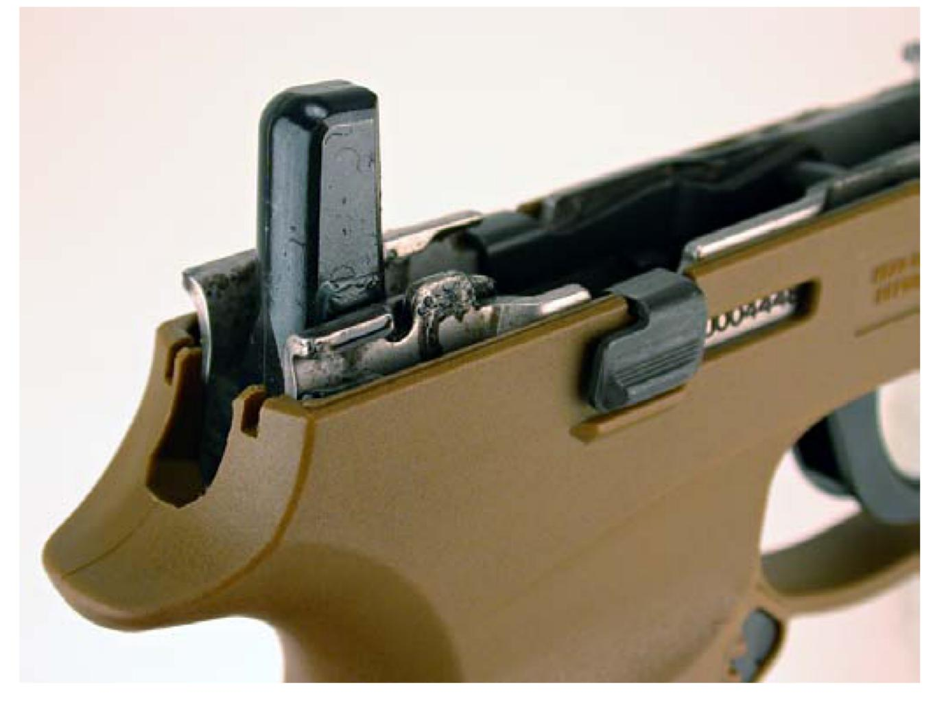
Our P250 pistol was a limited-edition model featuring a Flat Dark Earth grip module. But it was the action works, cloaked by the grip module, that was the serialized firearm. A window was cut into the side of the module to display the number.
