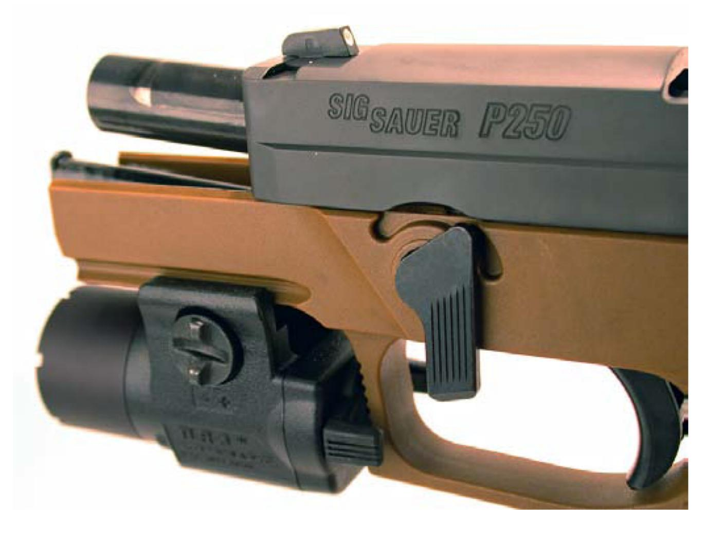
With the slide locked back and the latch rotated, the top end was ready to be removed. Note the polished area near the muzzle. That's just one point of lockup shared by our three pistols. There was plenty of room for a 90-lumen Streamlight TLR 3.
