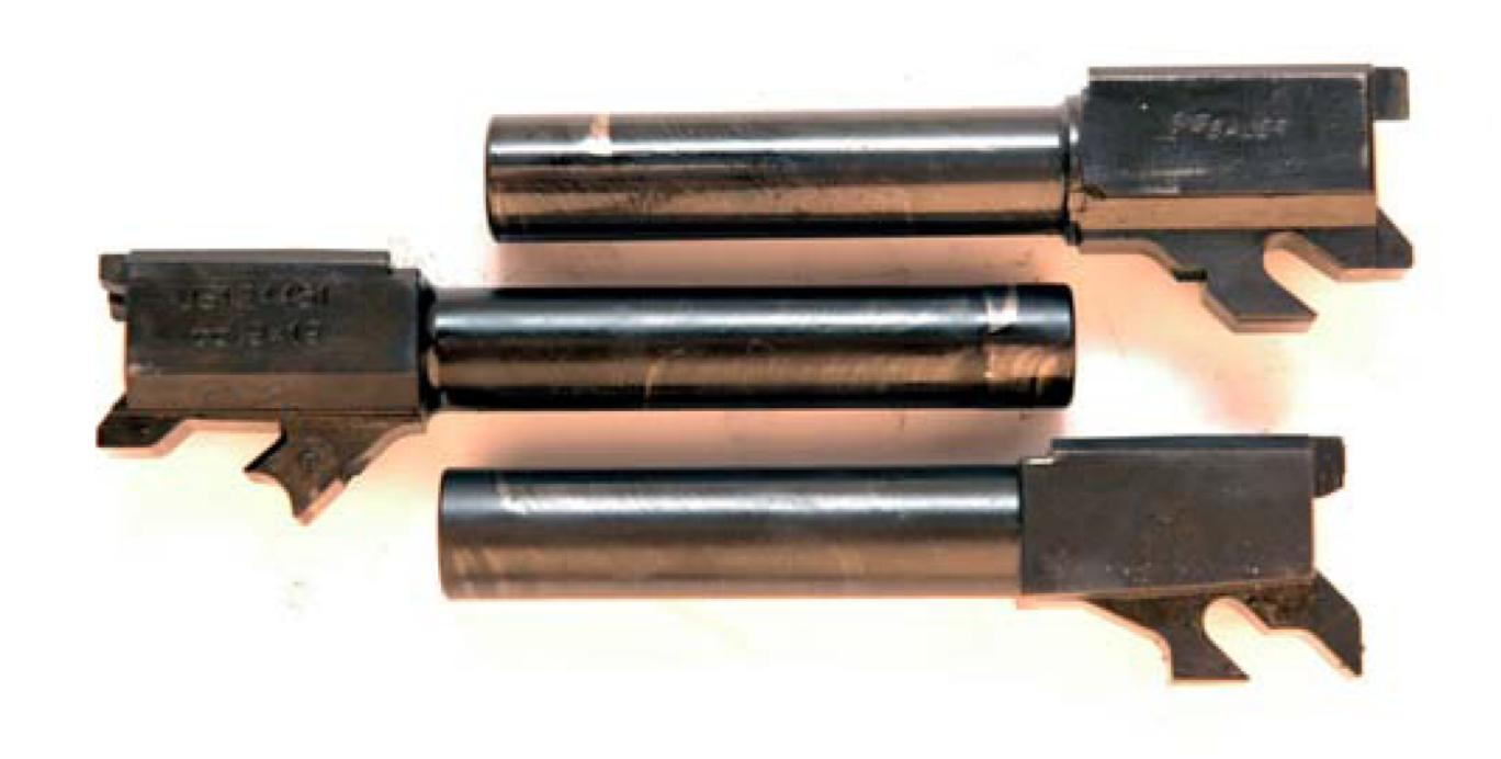
Side by side it could be difficult to tell one barrel from another. Top to bottom are the Sig Sauer P250, Springfield Armory XD, and CZ USA P-07 barrels. All three shared lock-up points and a ramp leading to the chamber. The XD's chamber was supported by a Sig Sauer–style locking block. After initial lubrication, all three guns ran without malfunction despite getting very dirty.
