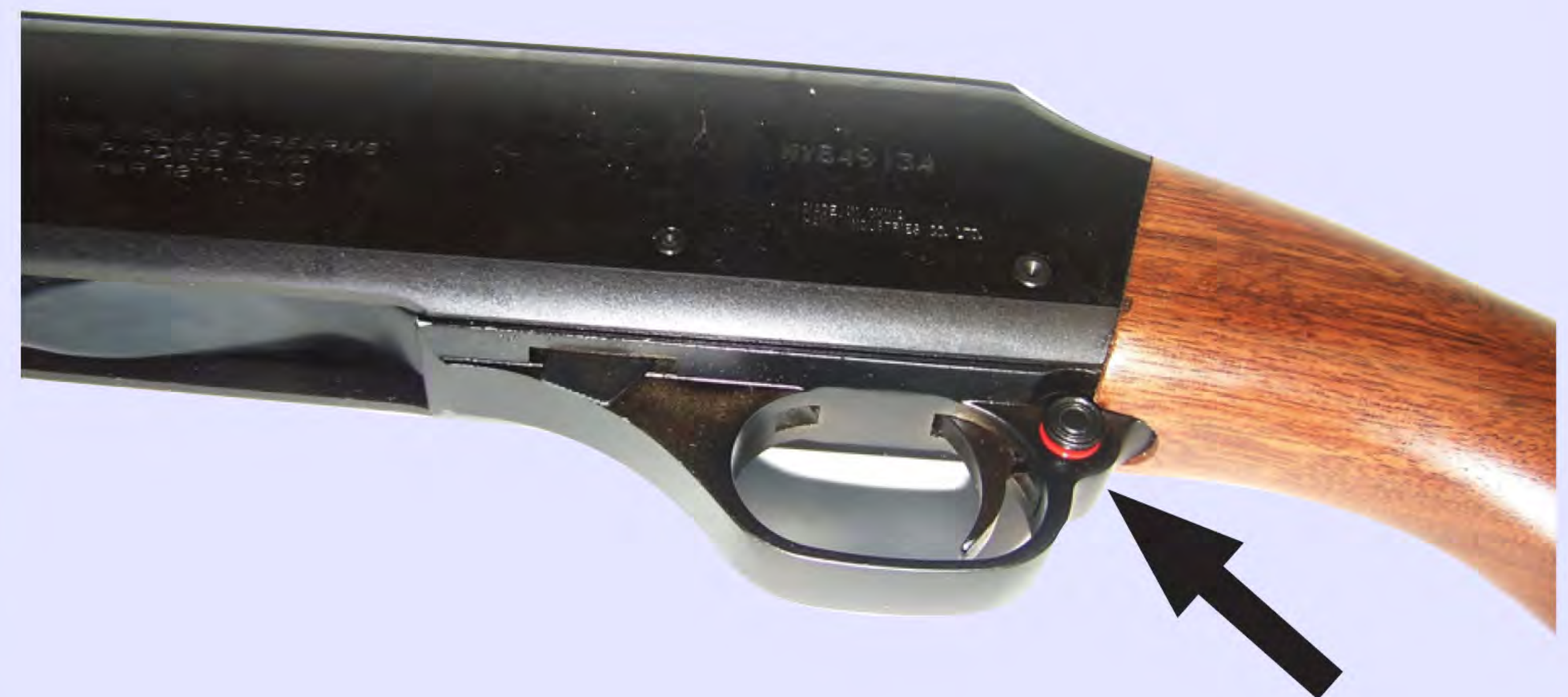
Above: The location of the cross bolt safety was ideal according to some of our raters. It certainly beat the Maverick.
