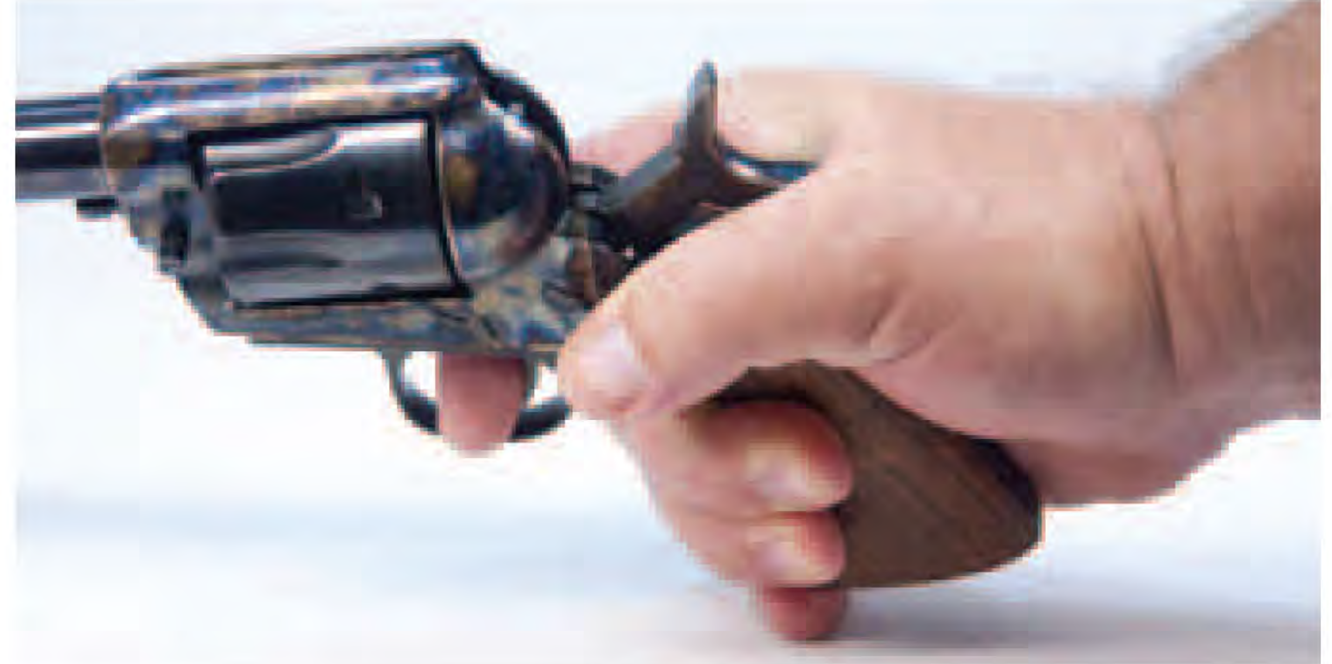
Above: Again with the hammer bite, this time on the Rough Rider. We know grasping lower on the grip solves this, but it also allows the muzzle to rise more on recoil. We want both control and comfort. Bottom: super-sharp edges on the hammer will draw blood.
