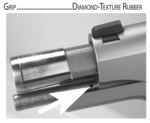
The lock-up point for the bull barrel was closest the muzzle. Removing material behind this point made the barrel more nimble as it moved in and out battery. The small hole in the full-length guide rod was for seating the takedown pin used to capture the recoil spring.
