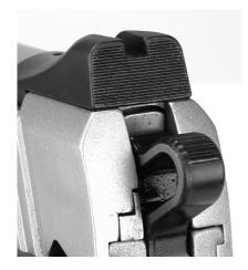
Both sights were grooved to reduce glare. They were snag-free and target grade. Blacking the outside of the hammer also helped reduce glare.
