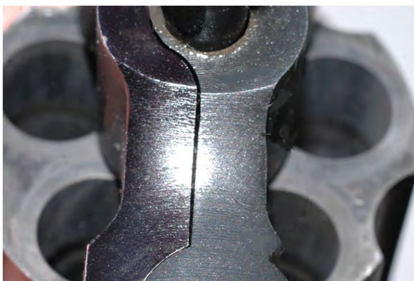
Above: The Centennial was pretty tight at the crane when we pressed the cylinder sideways.
