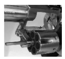
With an extra detent located in the crane, there was no lack of strength in the superstructure of the Redhawk.
