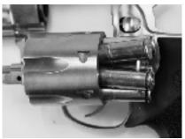
Above, left: Our main problem with the Redhawk was getting it to cycle. We think this was caused by the cylinder stop (arrow) failing to stay locked. This put the ratchet out of position. Above, right: We also had difficulty ejecting
