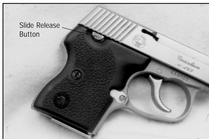
Left: Depressing the NAA Guardian's slide release button allows the slide to be removed. Right: The Seecamp LWS-32's slide is released by inserting a pin punch into a hole in the left side of the slide and depressing the slide retaining plunger.
