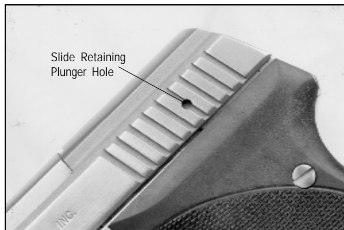
Left: Depressing the NAA Guardian's slide release button allows the slide to be removed. Right: The Seecamp LWS-32's slide is released by inserting a pin punch into a hole in the left side of the slide and depressing the slide retaining plunger.
