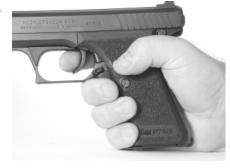
When the gun runs dry and locks back you release pressure to the front strap, insert the mag, squeeze the grip again and the gun immediately returns to battery. This is an advantage because you can shoot the gun dry to get full
