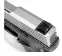
The Sigma's fixed rear sight was a Novak-style blade that aided in providing a clear sight picture and was very snag resistant. It was dovetailed to the slide and could be drifted for windage corrections.
