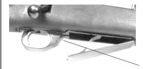
The Howa Model 1500 Lightning's magazine floorplate release was a pivoting lever-shaped catch that was partially recessed into the front of the trigger guard. The release worked stiffly.
