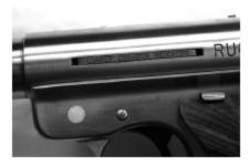
Above: The Mark III's loadedchamber indicator shown in the loaded position. We found it stuck out so little, and displayed so little warning orange, that the indicator could be easily missed.
