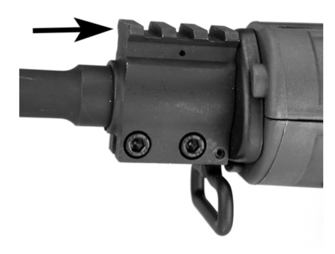
The Armalite featured a Picatinnyrail gas block (arrow). This gave the operator several options regarding choice of front sight or mounting accessories, such as lights or lasers.
