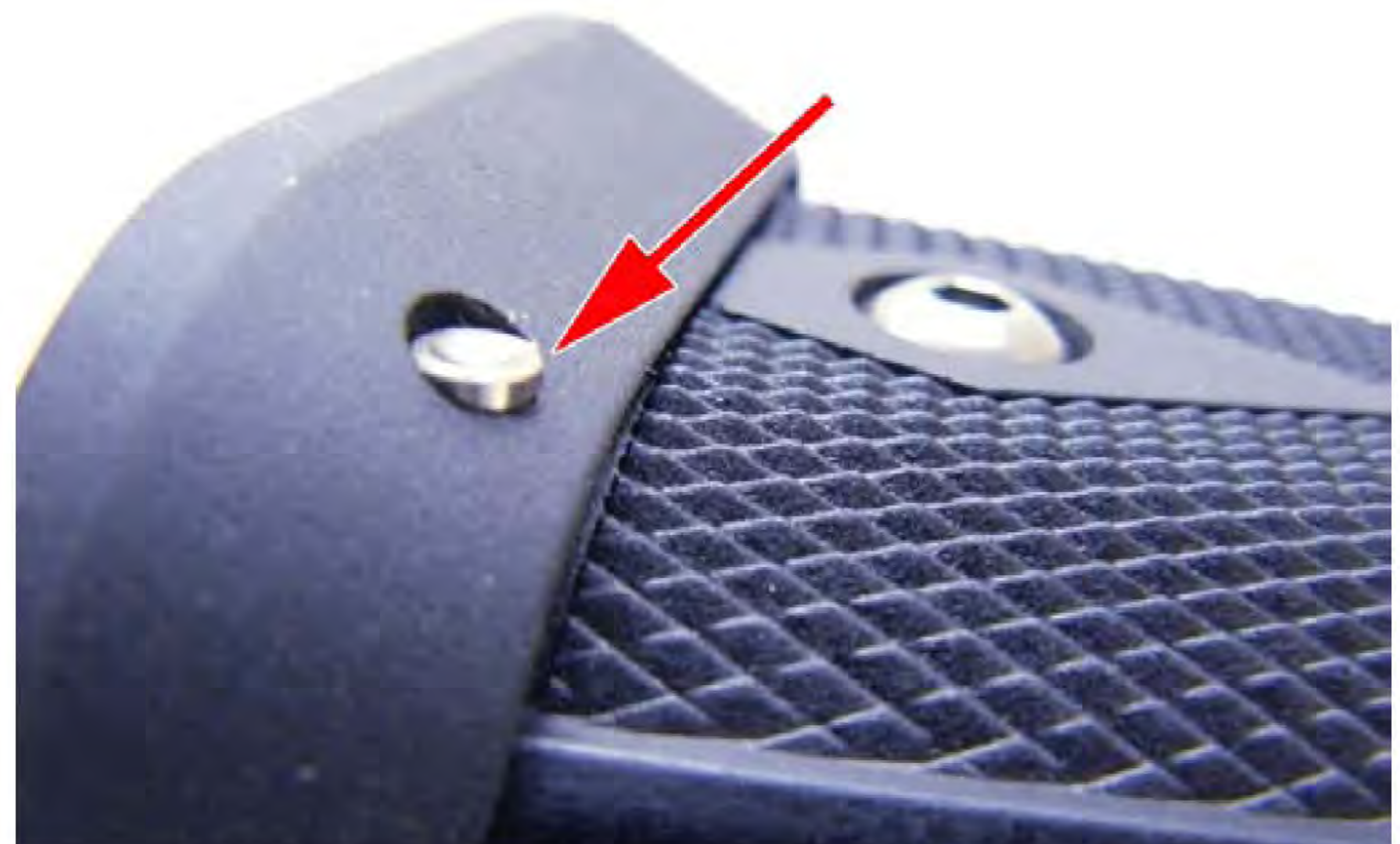
This rivet holding the mag well in place (arrow) was not flush inside the grip, and it bothered our left-handed shooters.
