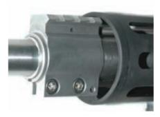
The circular aluminum forend simply stopped short of the gas-port block. The thick barrel got thicker from the port to the receiver. This was a heavy rifle.
