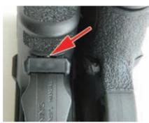
The H&K's magazine latch is fast and positive; however, one rater did not like seeing the internal spring behind the magazine release (arrow).
