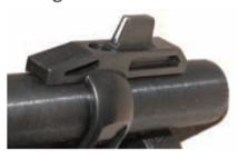
Above: The Henry's large rear aperture sight was fully adjustable for windage and elevation. It's locked by two opposing screws in the sight base. A smaller aperture that could be removed would be an improvement for some folks. Right: The white line is a groove in the rear face of the front sight blade. The blade is integral with the base and the barrel band. Remember that if you lower it by filing.
