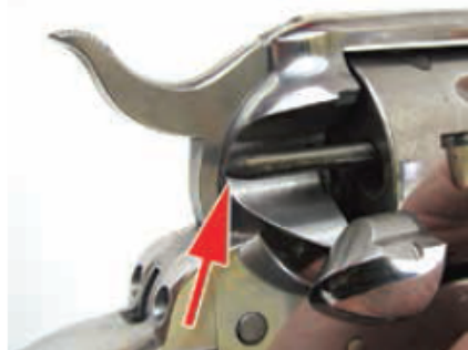
The Ruger's hammer at full cock did not leave a lot of room between it and the backstrap. We had the same problem on the Frontier revolver.
