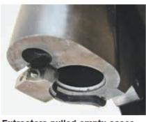
Extractors pulled empty cases or shells from the chamber. Note the plungers to hold the rimless 222 Rem. cartridge.
