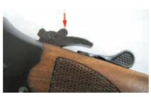
To choose which barrel fired first, the shooter toggled the small button on top of the hammer.
