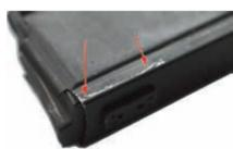
The arrows point to bare metal on the edge of the magazine, caused by the poor flt. All the magazines tried were too tight.
