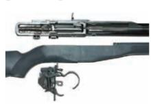
We slipped the metal out of the stock to have a peek inside. Pulling down on the trigger guard lets you remove the match trigger group, and then the rest lifts out. You can remove the bolt easily if desired.
