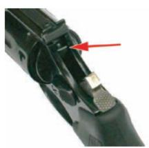
The transfer bar in front of the firing pin is coming into its fully upright position here.
