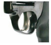
The trigger was wide and smooth — especially welcome with the 12-pound DA pull. Single-action trigger pull, 3.5 pounds, was better than the Ruger's.
