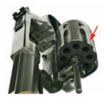
Note the front of the cylinder is chamfered to knock off that sharp edge. Also, that's a lot of steel for the rimflre 22 round. It could be made of another material or trimmed down to save weight. Inset: The ejector spewed out empties clear of the cylinder.
