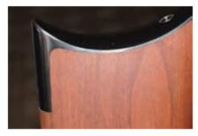
We've seldom seen inletting like this. This is essentially flawless fitting of metal to wood, whether done by computer (most likely) or by hand.
